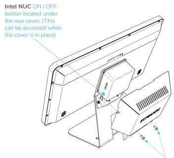
To remove the rear cover and access the NUC, unscrew the two fasteners using a 4mm allen key.
