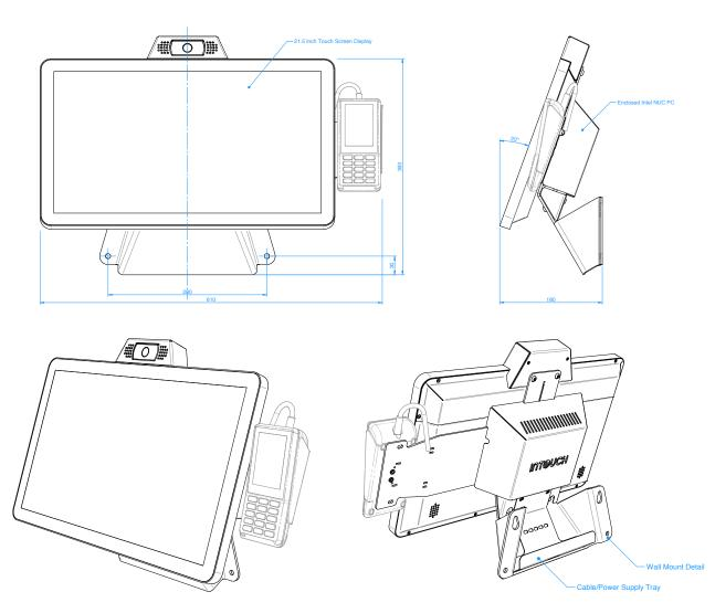
NOTE: Cabling & external power supplies not illustrated. Illustrated model includes peripheral devices.
