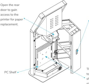
To access the inside of the kiosk. Unlock both key locks and use the handle depicted to open the door. (You may need to slighlty lift the door when opening)
