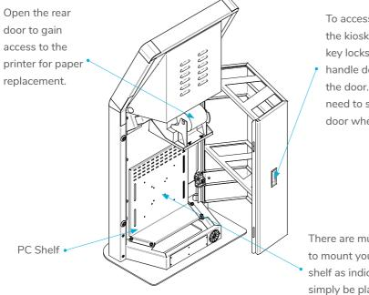
To access the inside of the kiosk. Unlock both key locks and use the handle depicted to open the door. (You may need to slighlty lift the door when opening)
