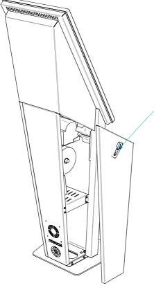
To access the inside of the kiosk, press the release button on the latch making sure the mechanism has been unlocked. Remove the door as shown in the image.
